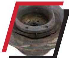
Torn strut insulator
