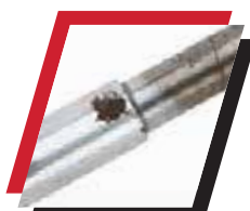
Damaged piston rod
